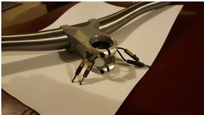
I want the cables to run under the grips and inside the handlebars, so this is how it should look like:
