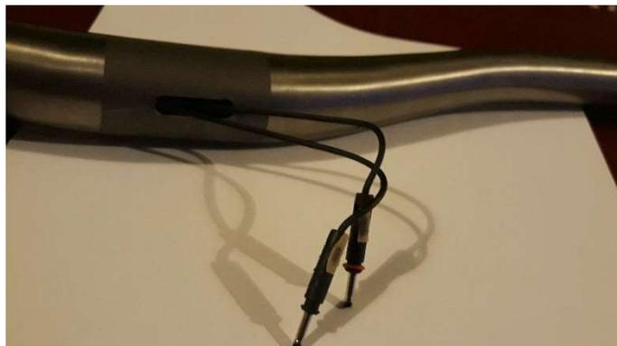
Now, I have a 2 bolt stem (Intend), so I need to put the stem in the handlebar at this point before inserting the other pair of cables.
