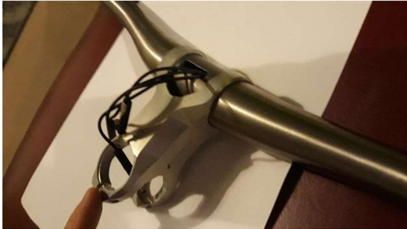
We pass the cables through the gap and carefully turn the handlebar to its final position. Obviously, this is way easier if you have a 4 bolt stem.
