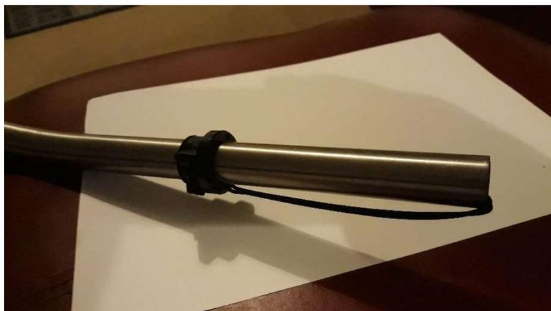
Now we just need to connect the cables to the Blipbox. Note that I had to modify the Blipbox so it fits inside the stem. A good amount of time went into carefully sanding the edges until it fits. Of course, this will void the Blipbox warranty, so be very careful not to sand too much!!
