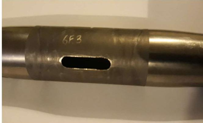
Drilling a hole at the back of the bars seems like a crazy idea, but I have been using this handlebar for almost a year with no signs of fatigue. I am 70kgs and ride Trail and Enduro style. For heavier riders and other disciplines like DH, it's probably better to get a handlebar with holes already. Zirbel, FSA and other companies make them, check them out.
